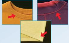
You simply change parts to perform other operations. The machine can perform covering, hemming and binding operations in addition to basic sewing.
