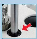
New type of oil-seal in the top of needle bar bushing.
