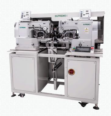
适用于风帽衬、运动休闲服饰类,腰绳及帽绳的车缝。自动送料、切料、塞绳头、套结、收料一次性完成,**7秒/根绳头**。Rope head knot machine Suitable for wind cap lining, sports and leisure clothing category, waist rope and cap rope seams. Automatic feed, cutting, plug rope head, tie, collection one-time completion, 7 seconds / root rope head.
